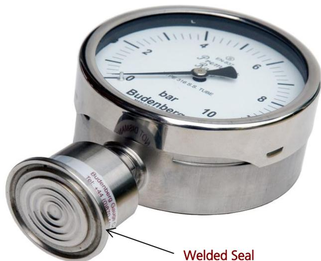
Budenberg weld a 316 stainless steel diaphragm to the stainless steel upper flange. This flange matches the coupling and enables the gauge to be taken off plant for cleaning. Crevice free construction reduces the risk of food traces being harboured and creating a health risk for food production.
